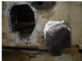
Hole in engine and insert piece
