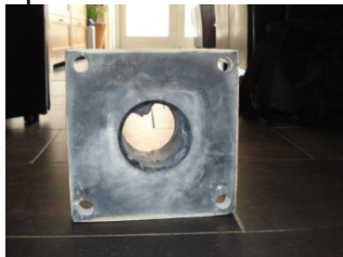
Flange before treatment
